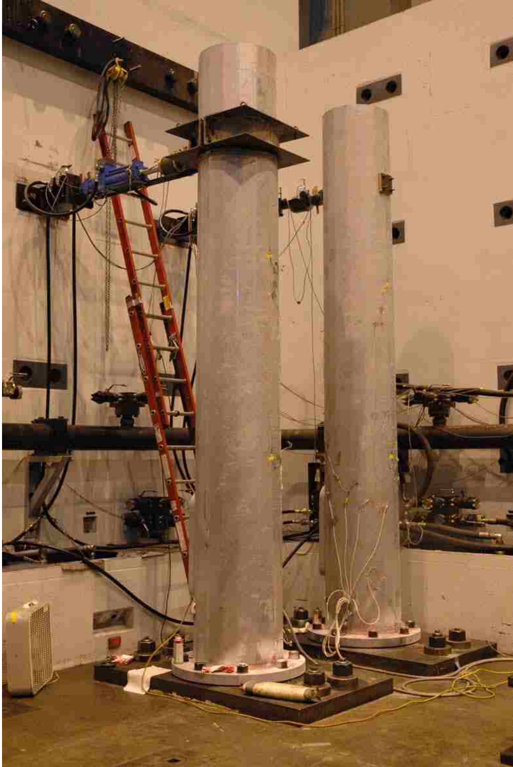
Figure 18. Fatigue testing setup at ATLSS
